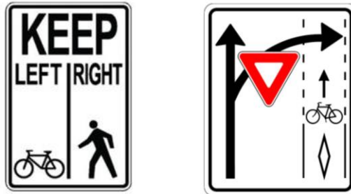
Figure 12. 'Pathway Organization' sign (a) and 'Turning Vehicles Yield to Bicycles' sign (b)
