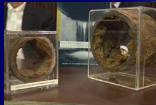
Deteriorating cast-iron water pipes -- similar to those still in use in some Ontario municipalities.
